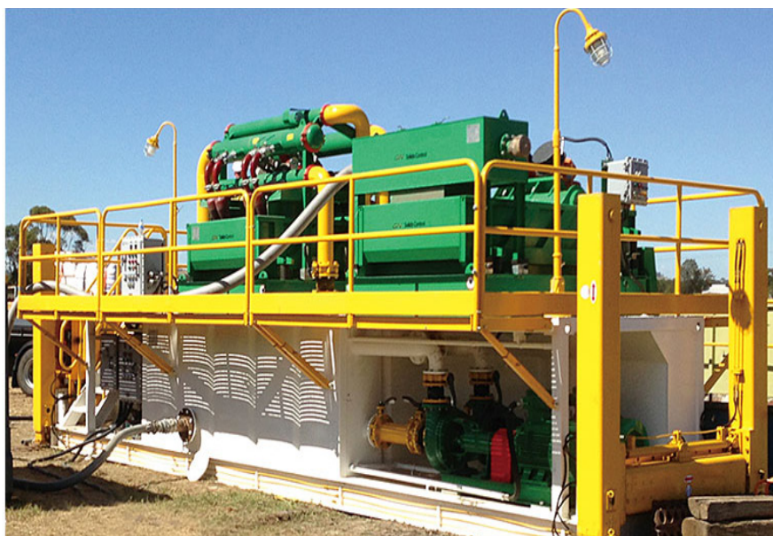
Fig. 4. HDD & CBM Mud Recycling System — GN Solids Control
